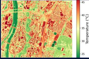
Land-Surface Temperature measured in the Bremen City Center using RAVEN.
